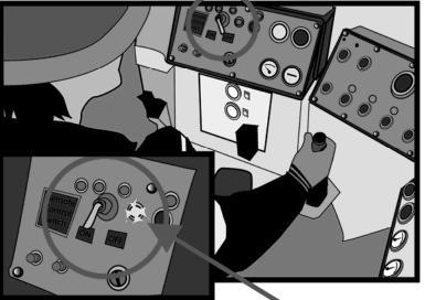
ensure the transmitter is non-functional before the operator approaches the equipment and takes over
