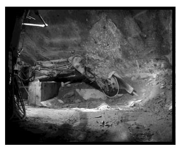
• A worker who was passing by a grizzly was struck by a piece of fly rock when the rock breaker shattered a piece of oversize material.
